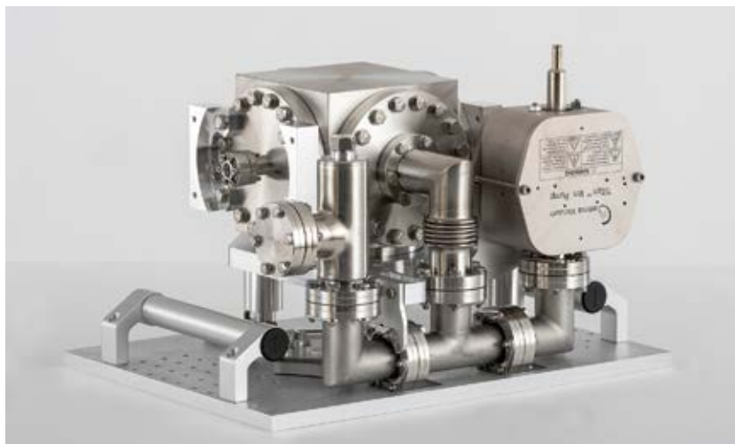
Fig. 3 Vacuum chamber containing the Fabry-Pérot cavity, with ion getter pump and incoupling viewport
