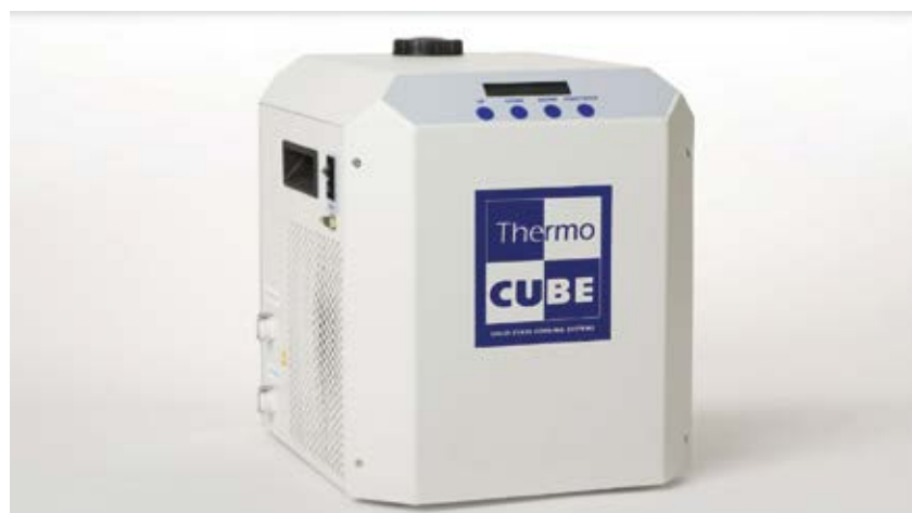
Fig. 2 Compact, benchtop recirculating chillers based on Peltier elements avoid the coolants required by compressor-based evaporation systems, but are less efficient – especially when cooling below ambient temperature is required. (Source: Solid State Cooling Systems)
