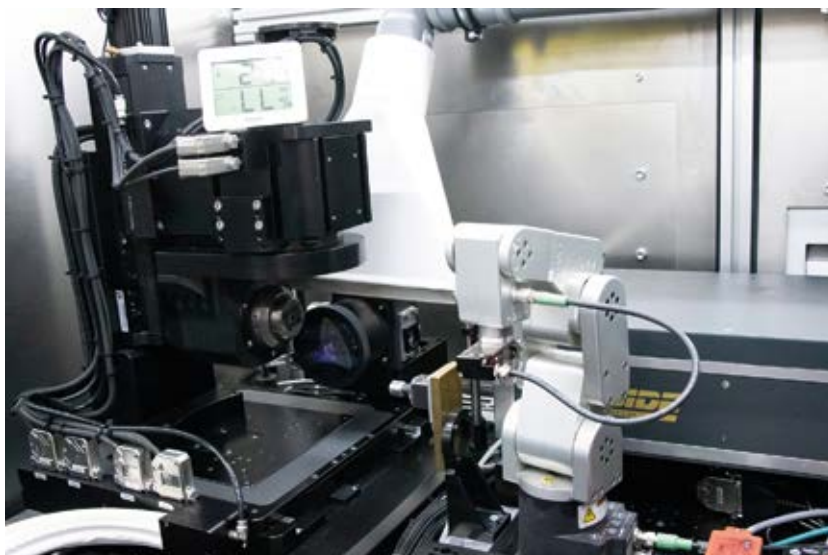
Fig. 2 Aerotech manufacturing system: A compact seven-axis system consisting of five swivel axes and two optical axes: the center of gravity is positioned exactly at the center of the machine, where a tool is lasered out with an integrated helix movement.
