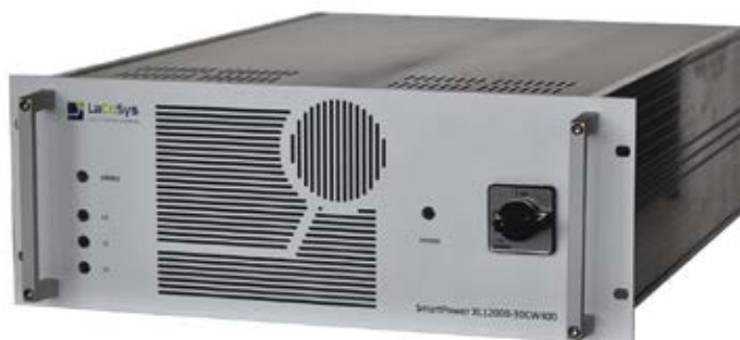
The Cotek AEK-3000 power supply takes on the role of a laser driver in the new LaCoSys burn-in test system. (Source: Systemtechnik Leber)
