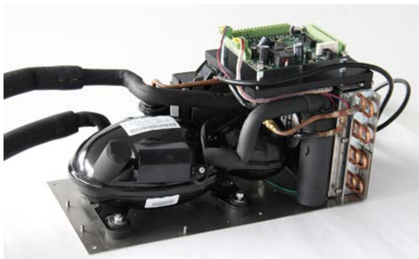
Fig. 5 Compressor unit for cooling solutions with the two refrigerant hoses leading to the left, directly connected to a cold plate or a laser diode stack where the refrigerant is evaporated – with no water loop required (Source: AMS Technologies)
