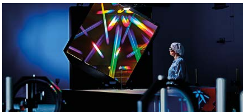
The large-scale interference lithography setup at the Fraunhofer Institute for Solar Energy Systems ISE (Source: Fh. ISE)
