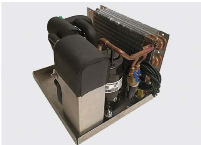
Fig. 3 Integrated cooling solutions based on a miniature 24 V DC rotary compressor with inverter fit into a space as small as 20 × 20 × 20 cm and deliver 450 W of cooling capacity for laser cooling (Source: AMS Technologies)
