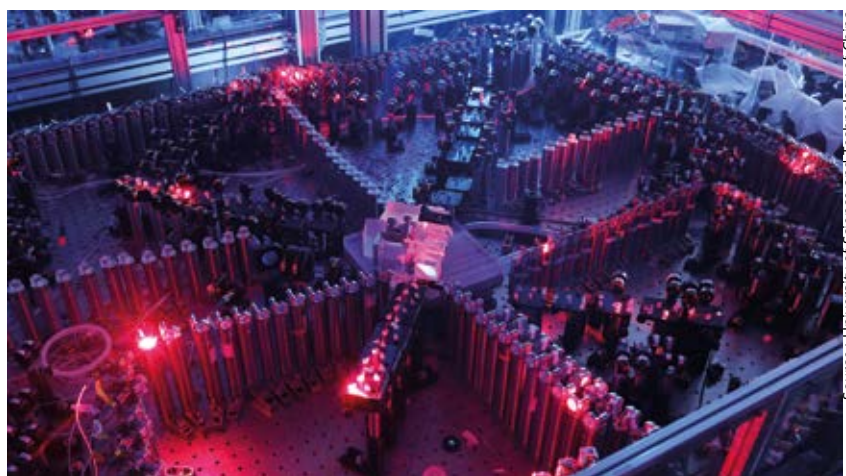
Optical structure of a quantum computer in a Chinese laboratory. With more than 70 photon qubits, this was able to demonstrate quantum superiority over a conventional computer when used for a special task.
