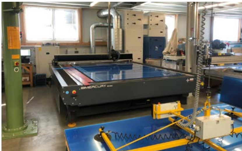
▲ The FilterCubes are directly connected to the lasers and provide high-performance extraction at the very place where the dust and fumes are generated.
