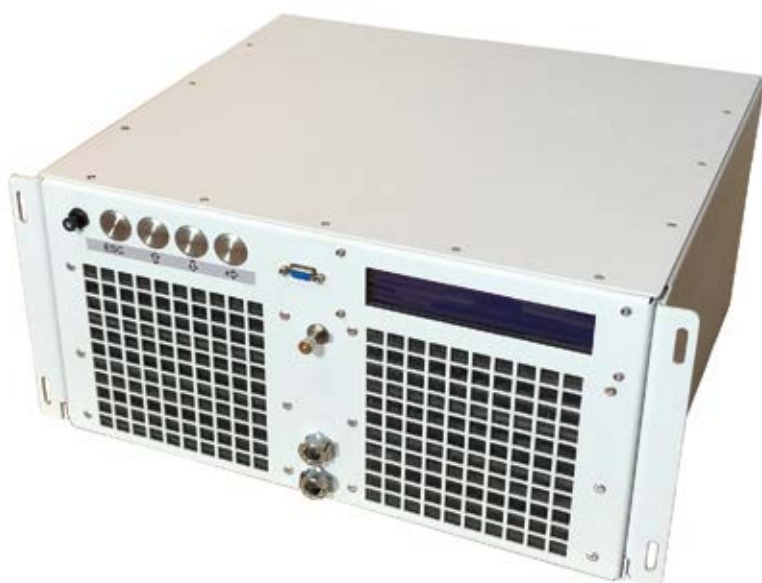
Fig. 4 Two miniature, speed-controlled compressors in a 5U rackmount system can provide up to 1600 W of cooling capacity (Source: AMS Technologies)
