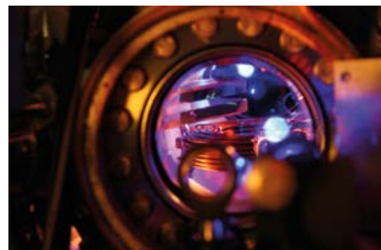
Blue fluorescing cloud of atoms that have been laser-cooled to milli-Kelvin temperatures in the PTB's strontium lattice clock. (Source: PTB)
