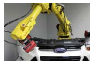
Gap and flush measurement with Perceptron technology AutoFit (Source: Isra Vision)
