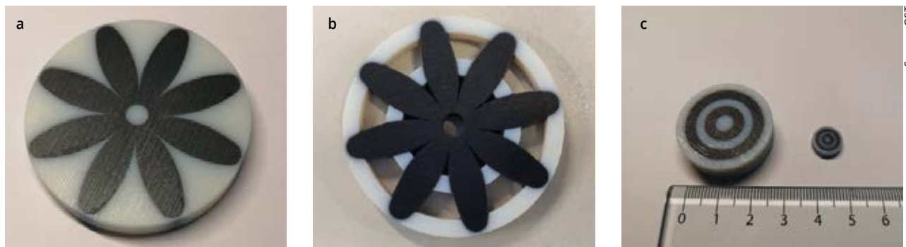
Novel GRIN polishing pads for synchro speed polishing are currently under investigation: (a) a full material synchro speed polishing pad (b) a lightweight synchro speed polishing pad and (c) a special, full material synchro speed polishing pad in two dimensions for lens diameters of 9 mm and 4 mm. Smaller pad dimensions are currently under investigation.
