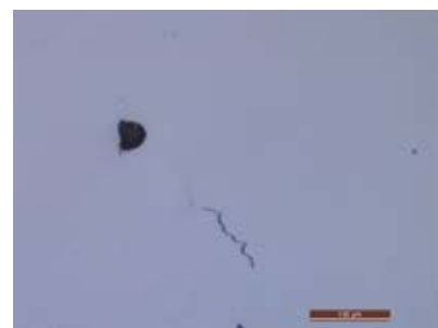
Fig. 3 Micrographic evaluation of samples made with the ring shape at different scan speeds; (left) ring shape – scan speed: 550 mm/s – \times 50 , (right) ring shape – scan speed: 690 mm/s – \times 200
