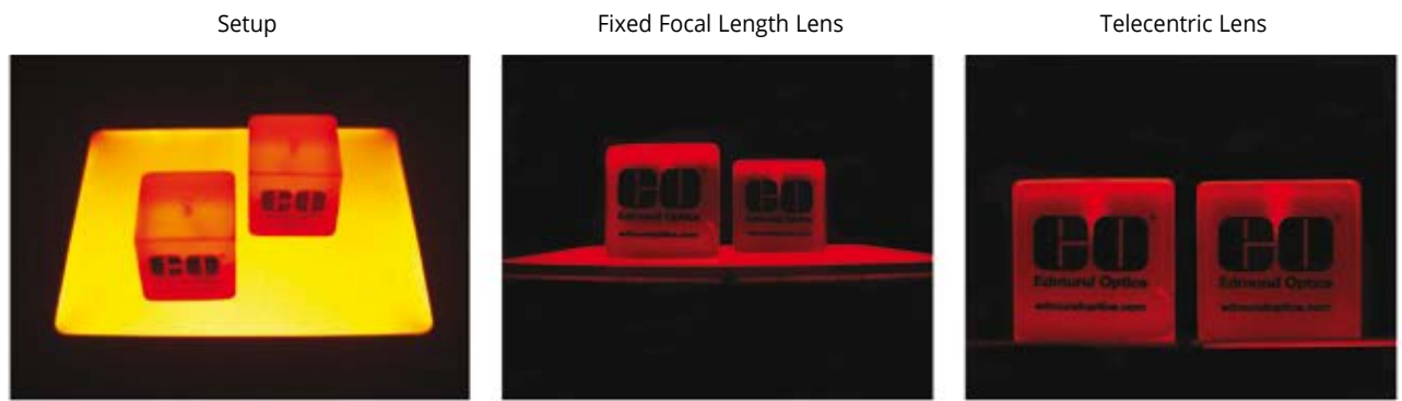
Fig. 1 Middle image: Due to the aperture angle of the fixed focal length lens, the right cube is imaged smaller than the cube of the same size that is closer to the inspection system. Right image: The same scene taken with a telecentric lens. Now both cubes are the same size.
