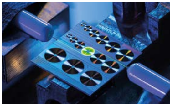
An erbium-doped waveguide amplifier on a photonic integrated chip. (Source: N. Ackerman, LPQM, EPFL)
