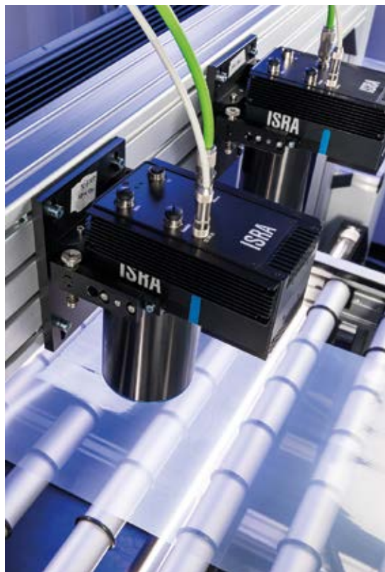
Isra Vision SMASH surface inspection system for plastic film material
