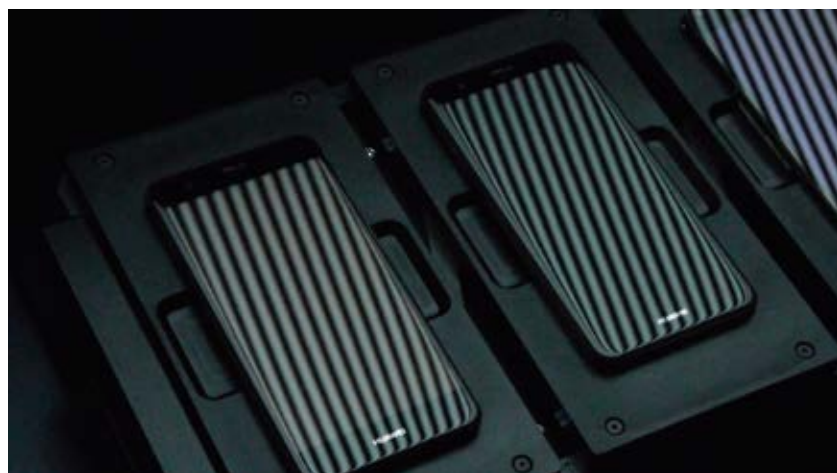
Deflectometric surface inspection of the end product
