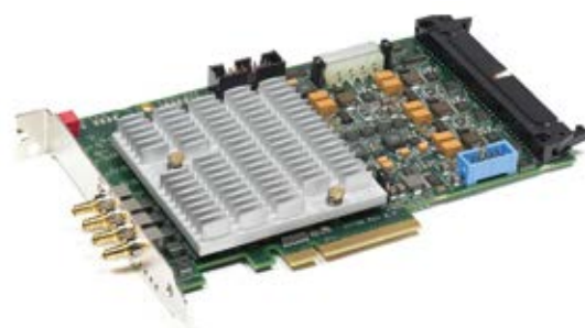
Above: BitFlow Cyton CXP CoaXPress frame grabber Left: Schematic of the MS-BLIP system (Sources: BitFlow)
