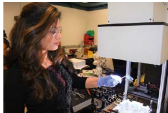
Nina Vaidya measuring the experimental performance of optical concentrators under a solar simulator that acts as an artificial sun. (Source: N. Vaidya)
