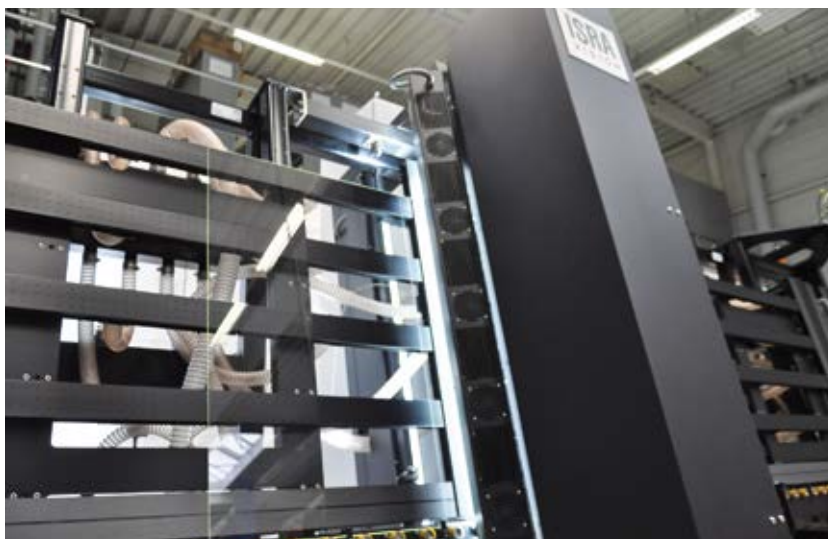
Isra Vision Flat Panel Master performing thin glass surface inspection for displays
