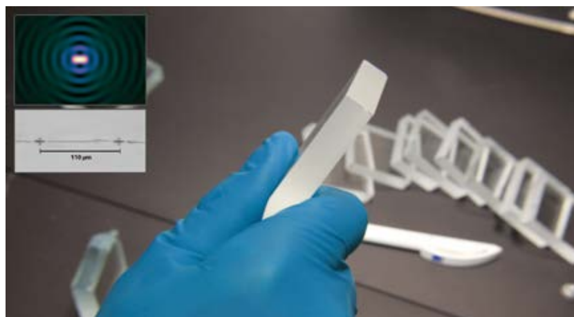
Fig. 2 Architectural glass with a thickness of 12 mm separated by multiple non-diffracting beams. The samples have been realized by TruMicro series ultrafast lasers, providing mJ-range pulse energies. The top inset shows the lateral intensity distribution for multiple Bessel-like beams. The lower inset is a reflecting light microscope picture top view of two laser modifications. The resulting intensity distribution enables the modification distance to be increased up to 110 \mu\text{m} [4].
