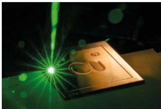
Laser materials processing of copper with a green laser (Source: BLZ, Cvecek, Kaufmann)
