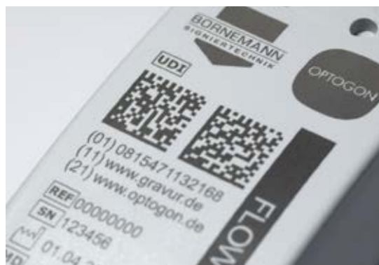
Laser marking of an individual UDI code on a plastic housing for the medical industry
