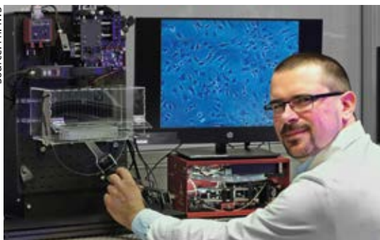
The new white-light laser source enables scientist Tobias Baselt to detect cell changes in real time.
