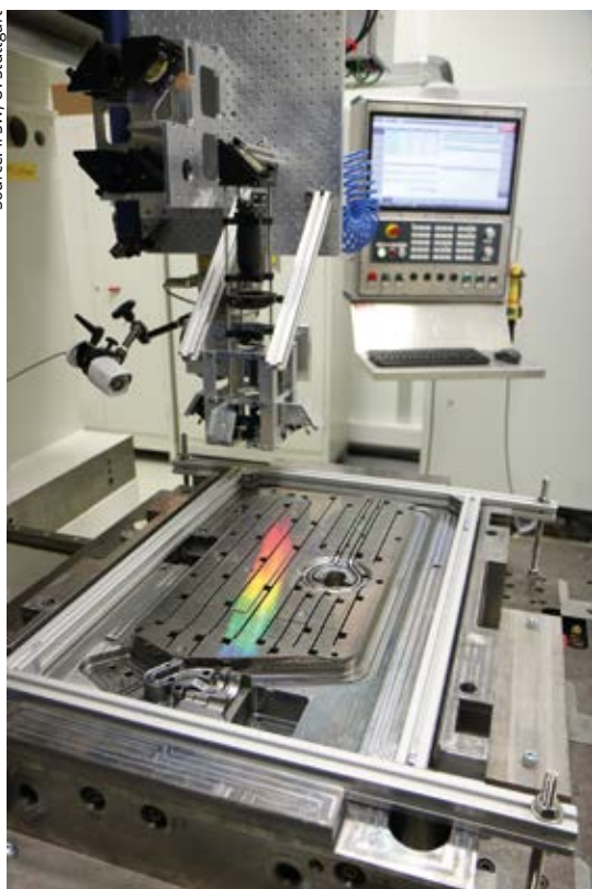
The Tresclean project (tresclean.eu) aims at developing high-throughput laser-based texturing for fluid-repellent and antibacterial metal surfaces
