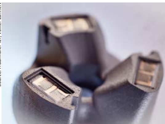
Fig. 5 LPBF-manufactured component with integrated sensors
