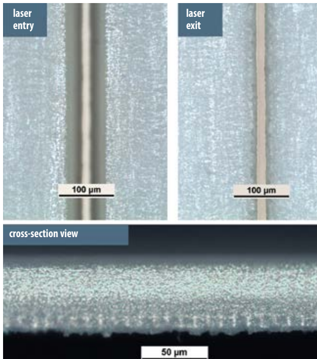
Fig. 1 Bare 50 µm thick LCP cut with Quasar UV80 laser. Entry (top left), exit (top right), and cross-section (bottom) views indicate excellent quality and minimal excess heating.
