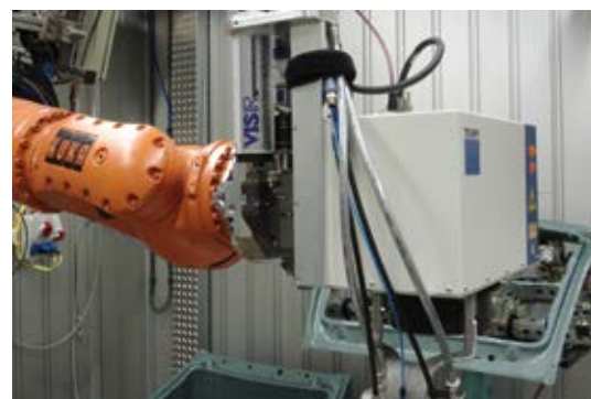
Fig. 4 A Trumpf PFO 3D with a Hema ICAM LASER camera on a KUKA robot (Source: Mercedes-Benz AG)
