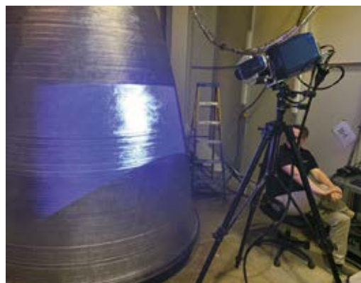
This part is scanned inside the DM3D printer using Hexagon's StereoScan Neo R16 structured light scanning technology. (Source: Hexagon)
