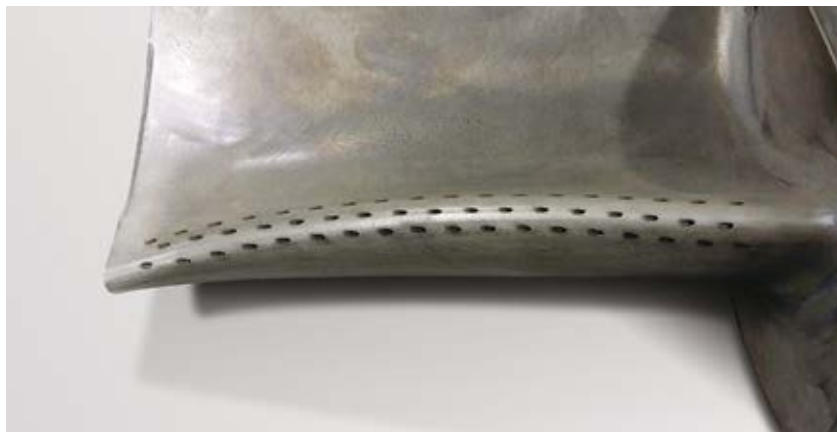
Numerous openings to the hollow interior of the blades in modern gas turbines provide cooling for the blade surface (Source: Synova)
