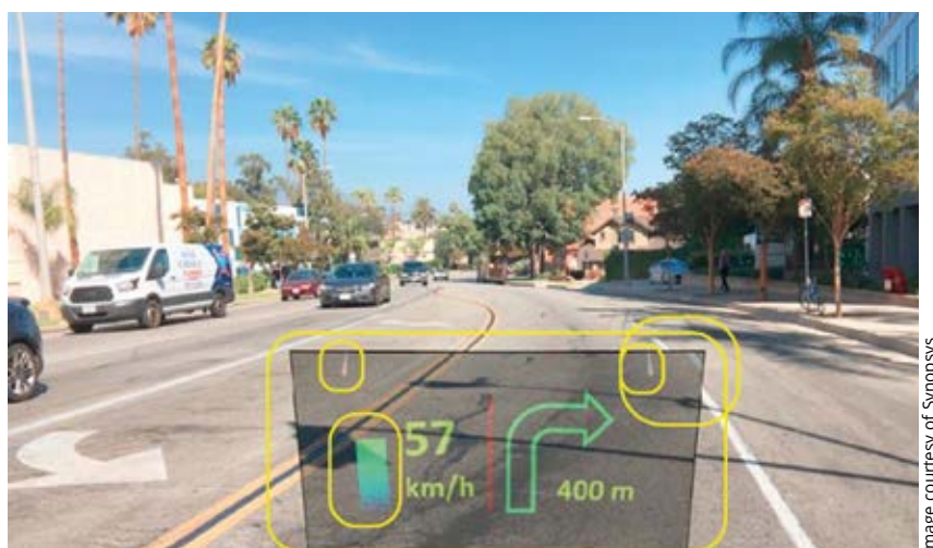
Fig. 12 Illustration of virtual prototyping using Synopsis LightTools software of a head-up display (HUD). The simulation shows different image non-imaging effects and allows the resulting image quality to be evaluated. The various parameters that can be seen (marked by yellow) are the see-through contrast and color on the highly lit background; the color uniformity (on the bar area); the see-through transmission (darker HUD beam splitter); the ghost images (white lines without corresponding lines on the scene); the prismatic deviation (white separation line appears 'broken')
