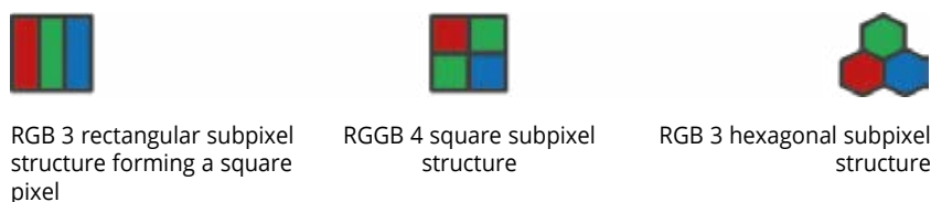
Fig. 4 Different types of microdisplay sub-pixel structure and arrangement. The different arrangements are related to the image Nyquist frequency resolution, which may differ for horizontal and vertical axes
