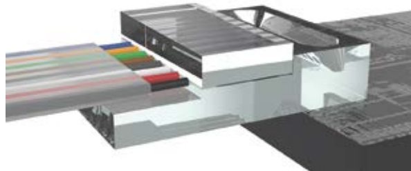
OptoCplrLT with fiber assembly, coupling to SiPh grating couplers (Source: Optoscribe)
