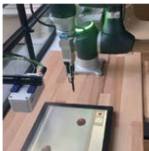
Live-ready AI conveyor belt sorting with a Framos D435e industrial depth camera
