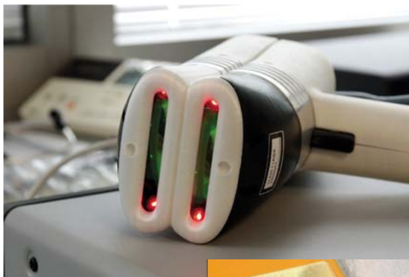
Fig. 2 A multibeam LDV demonstrator implemented in the H2020 CARDIS project (continued by the H2020 InSiDe project, inside-h2020.eu). The laser source is hybrid integrated on the PIC, based on micro-optical bench (MOB) technology. (Source: Imec).
