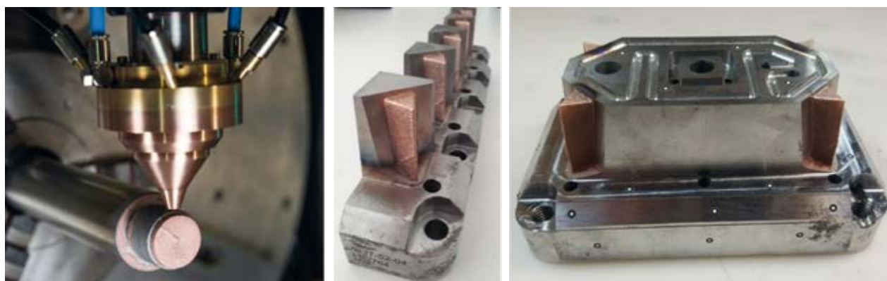
Fig. 7 LMD with a green laser to build up multimaterial mold inserts (pure Cu / steel 1.2764).
