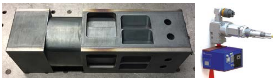
Fig. 9 Demonstrator with complex surface geometry, laser hardened with a TFC system from left to right in one continuous track, track width 45 mm (left); 3D drawing of the new TFC laser head (right).
