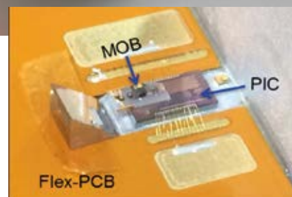
Fig. 2 A multibeam LDV demonstrator implemented in the H2020 CARDIS project (continued by the H2020 InSiDe project, inside-h2020.eu). The laser source is hybrid integrated on the PIC, based on micro-optical bench (MOB) technology. (Source: Imec).
