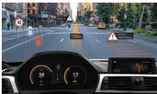
Infineon’s MEMS scanner chipset enables AR-HUD systems with minimum optical volume. (Source: Infineon)
