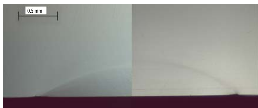
Fig. 5 Comparison of a standard (left) and AQW process (right) weld nugget (Source: Evosys)
