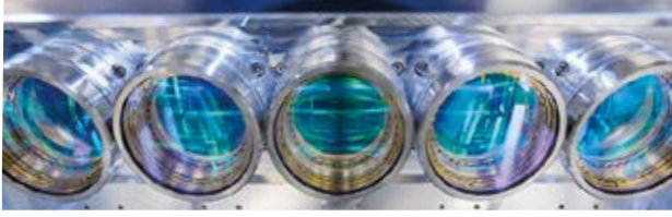
Optical system of a multiscanner LB-PBF system. (Source: Fh. ILT)
