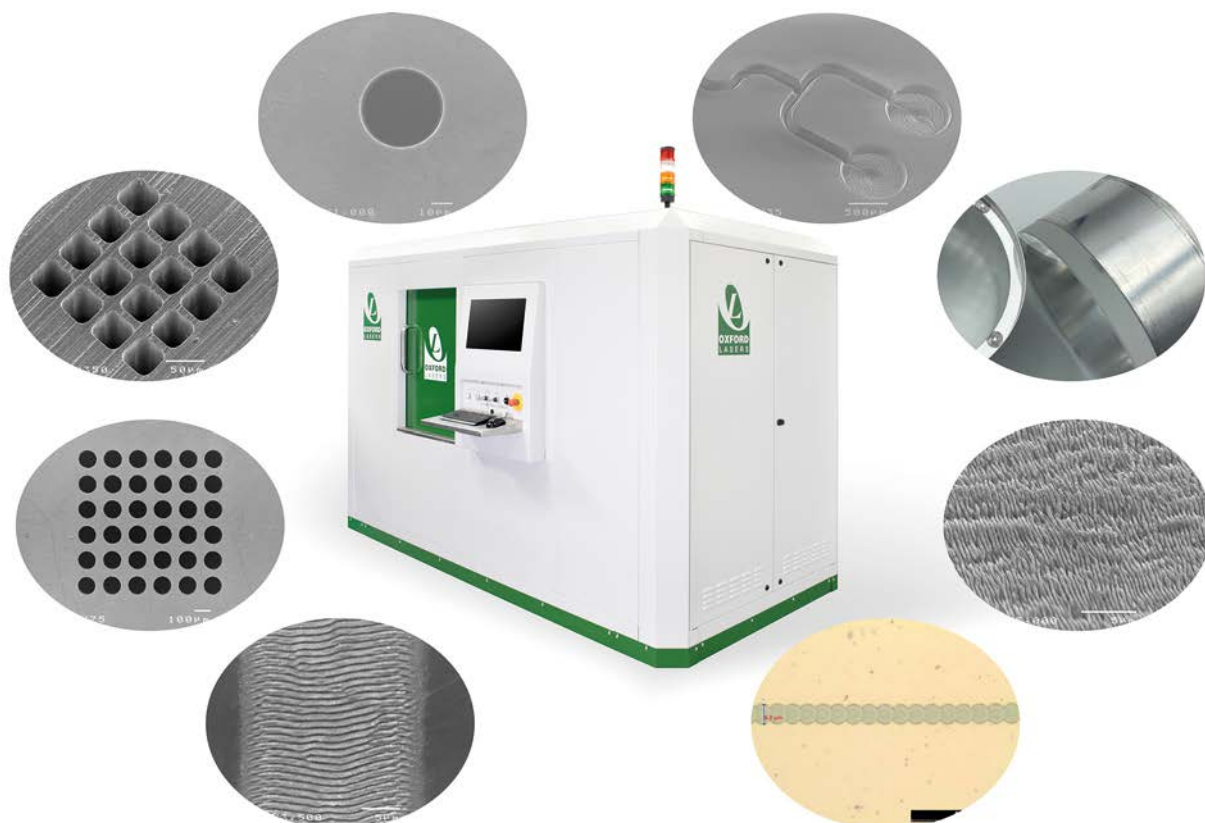
Fig. 4 Micromachining capabilities of Oxford Lasers. Images clockwise from top right: laser milling microfluidics in borosilicate glass, laser welding of dissimilar materials – BK7 glass welded to aluminium, laser surface texturing for controlled wettability (hydrophobicity), thin-film patterning – indium tin oxide on PET, surface texturing of stainless-steel channels, laser drilling 90 µm holes in polyimide, laser drilling 50 µm square holes in silicon nitride, laser drilling a 35 µm hole in molybdenum. Center image: an Oxford Lasers C Series industrial micromachining tool (Source: Oxford Lasers)
