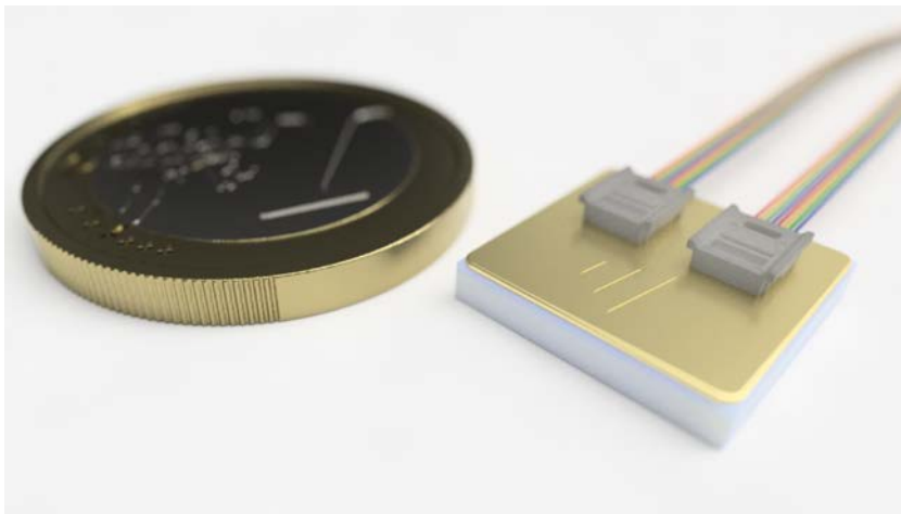
Co-packaged optics – silicon photonics transceiver design for high speed serial interconnects being developed through ESA ProtoBIX activity.
