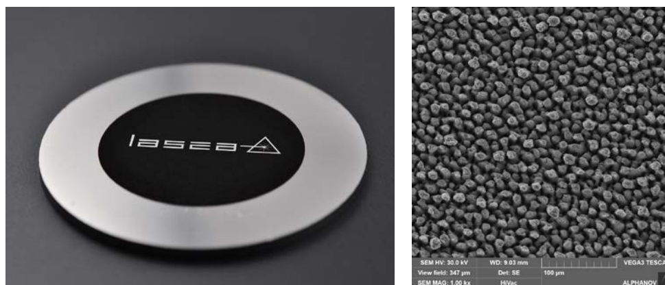
Fig. 2 Example of the micromachining capabilities of the Lasea company. Deep black texturing macro (left) and microscopic views (right) (Source: Lasea)
