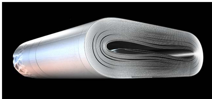
Delaminations, the detachment of the electrode windings or coatings, can be easily visualized with CT. (Source: Volume Graphics / Waygate Technologies)
