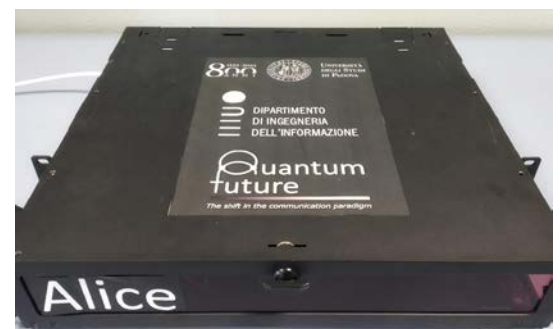
The entire transmitter for the new QKD system fits in a 19-inch rack enclosure. (Source: L. Calderaro, U. Padova)
