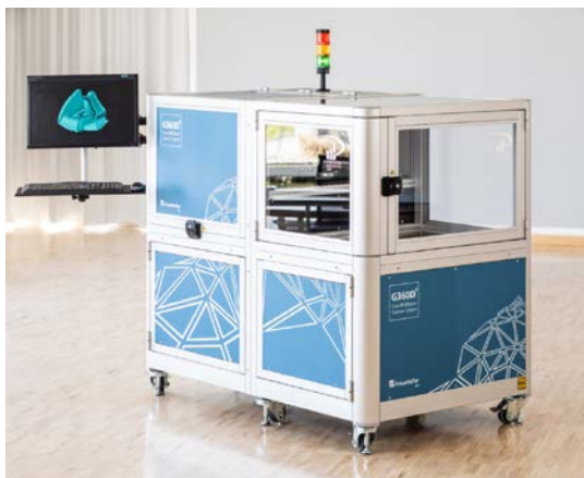
“Glass360Dgree”: First MWIR 3D system for checking Glasele in optics manufacturing (Source: Fh. IOF)
