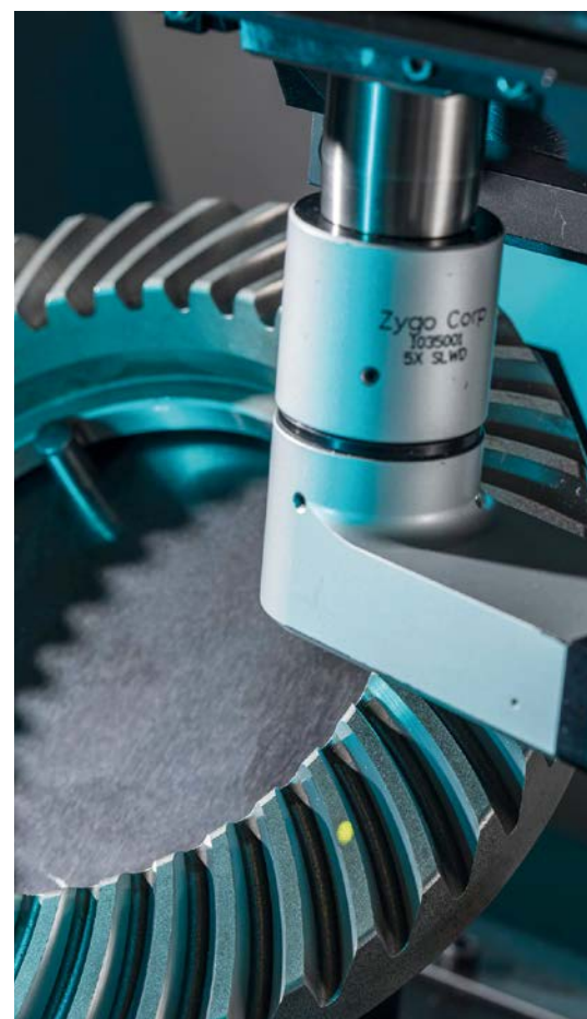
Fig. 3 Interference microscopy for measuring gear shape and texture
