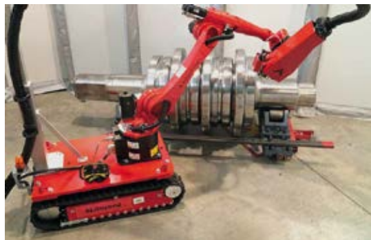
Laser hardening of a shaft using the mobile ALOHybrid configuration. (Source: Alotec)
