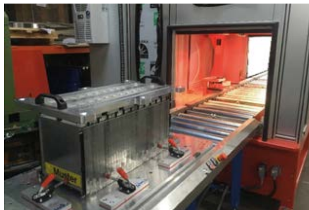
To win more power of the battery the electrodes has to combined by welded busbars. The advantage of laser welding is a short application of energy. This will reduce the warming of material.
