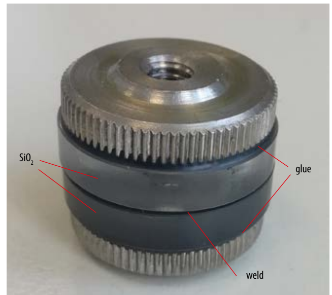
Fig. 2 Welded fused silica substrates glued to knurled nuts for tensile testing.
