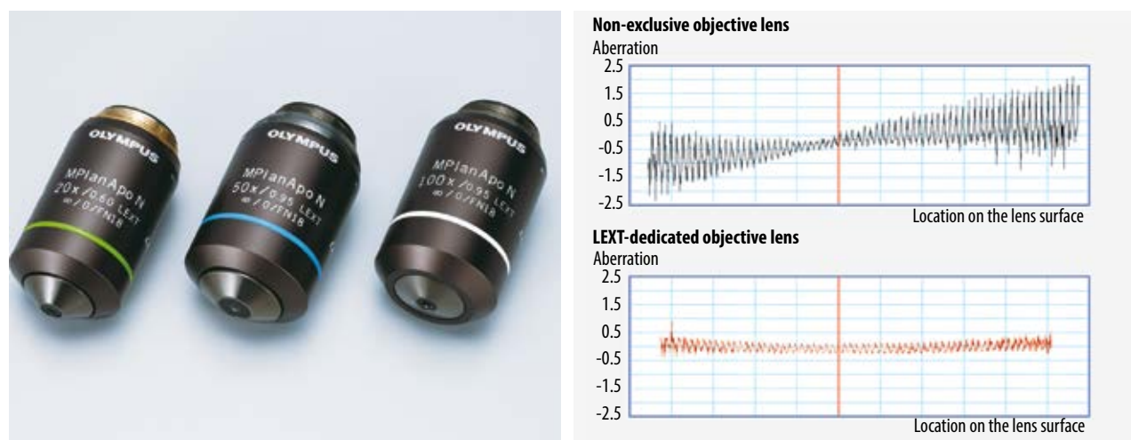
Fig. 8 Lens Performance comparison with objective lenses specially designed for 405 nm light. Left: LEXT-dedicated objective lenses, right: aberrations are highly reduced (orange curve) when using LEXT-dedicated lenses.
