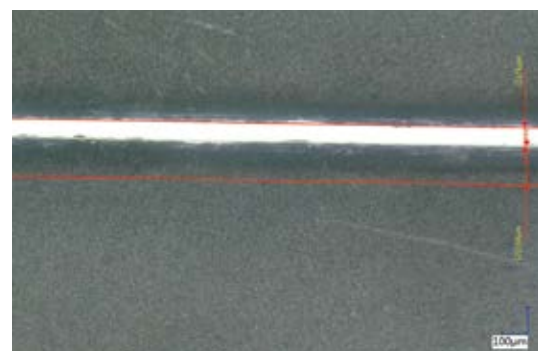
Deflection units can be used to generate battery foils quickly and precisely: Here, a cut edge of a cathode with lithium-nickel-cobalt-manganese oxide coating. (Source: Sonplas)
