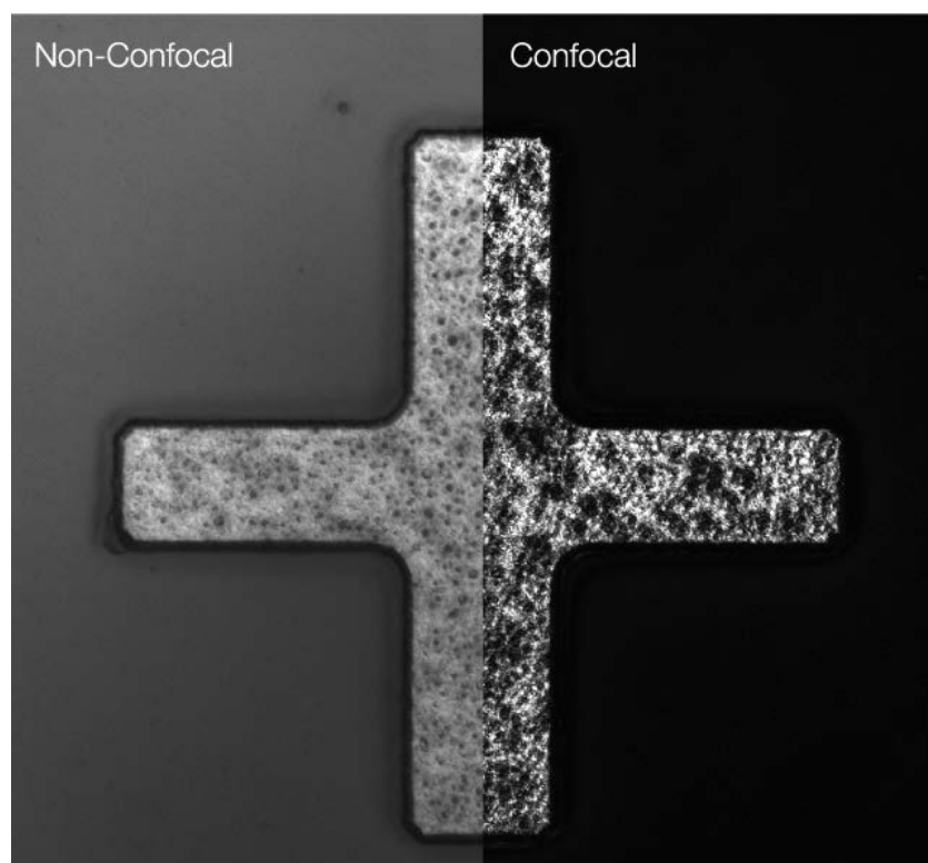
Fig. 5 Comparing non-confocal (left) and confocal (right) imaging (Source all images: Olympus IMS)
