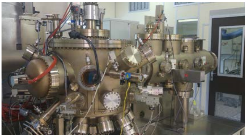
MBE technology – Almae's workhorse for photonic integration
