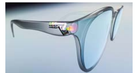
Silicon micromirrors project images and data onto the glasses. (Source: Oqmented)
