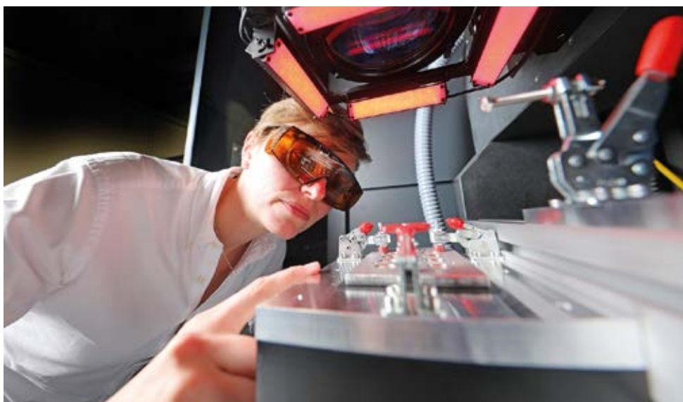
An employee from the Fraunhofer ILT in Aachen checks the settings of the scanner system. Below is a clamping device for a sub-module of cylindrical cells. (Source: Fh. ILT)
