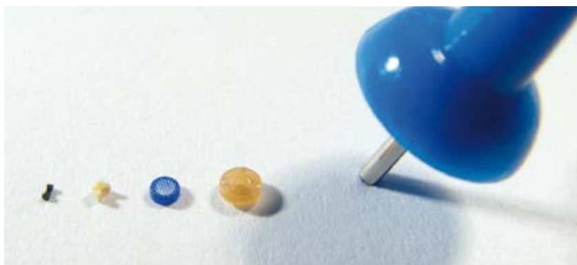
Fig. 3 Examples of micro injection molding. Smallest part on the left is a mineral-filled LCP under 1 mm in total size. The largest part is a 2 mm PEEK driver for a medical device. The blue part is 1.5 mm nylon component with an overmolded fabric mesh. The tan part is a LCP fiber alignment wedge.
