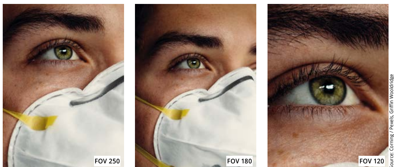
Fig. 2 Effect of the field of view (FOV) on the size of the iris on a detector at constant distance
