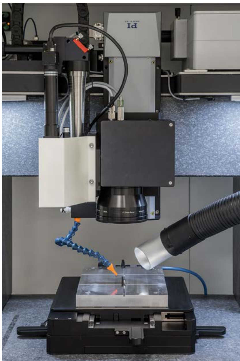
Fig. 4 Multiaxis setup comprising linear motor-driven Model 731 XY planar stages (8 × 8" travel) and screw-driven Z stages from Physik Instrumente, and a galvanometer scanner from Scanlab for laser marking precision components at high speed. (Source: PI)
