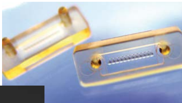
Fig. 2 Fiber optic connector, Ultem (PEI), 12 Ø 250 µm lenses with a 250 µm pitch between lenses with a ±2 µm non-accumulative positional tolerance.
