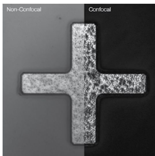
Fig. 5 Comparing non-confocal (left) and confocal imaging (right)
