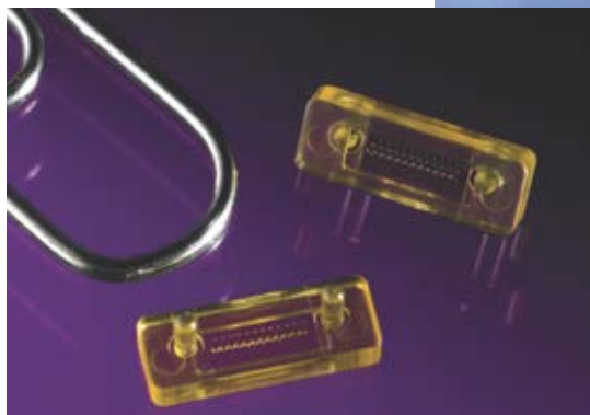
Fig. 2 Fiber optic connector, Ultem (PEI), 12 Ø 250 µm lenses with a 250 µm pitch between lenses with a ±2 µm non-accumulative positional tolerance.
