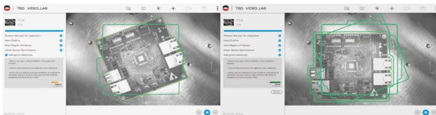
Fig. 2 The second AI module is used for detection and alignment. It allows the system to recognize the parts it sees in a live video stream and identify the best moment to capture an image. This image will be used to perform the last task: defects inspection.
