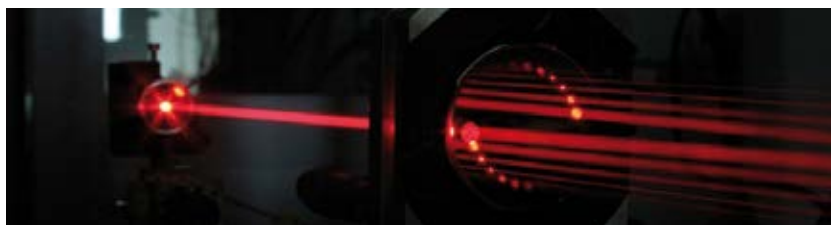
An extremely sensitive, yet simple optical method for detecting formaldehyde: the approach is based on multipass spectroscopy, which introduces a laser through a small hole in a mirror. The laser light then bounces back and forth between mirrors, creating interaction lengths with the sample that are tens or hundreds of times the length of the cell. (Source: M. Winkowski, U. Warsaw)
