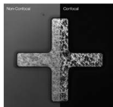
Comparing non-confocal (left) and confocal (right) imaging. (Source: Olympus)
