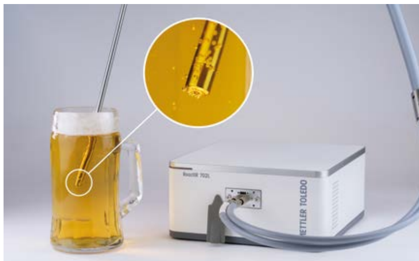
Fig. 2 Test your beer with IR-fiber spectroscopy. (Courtesy of Art Photonics)
