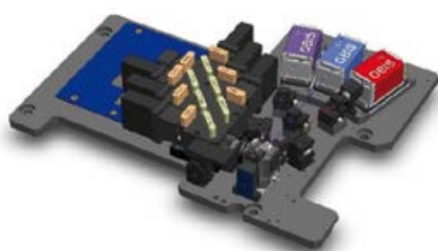
Fig. 3 The use of several lasers in a single instrument involves numerous adjustable optomechanical components which must all be specified and aligned by the instrument builder (left; source ACEA Biosciences). A self-contained multiwavelength light engine with independent adjustment of each wavelength can replace all these standalone lasers and optomechanics (right).
