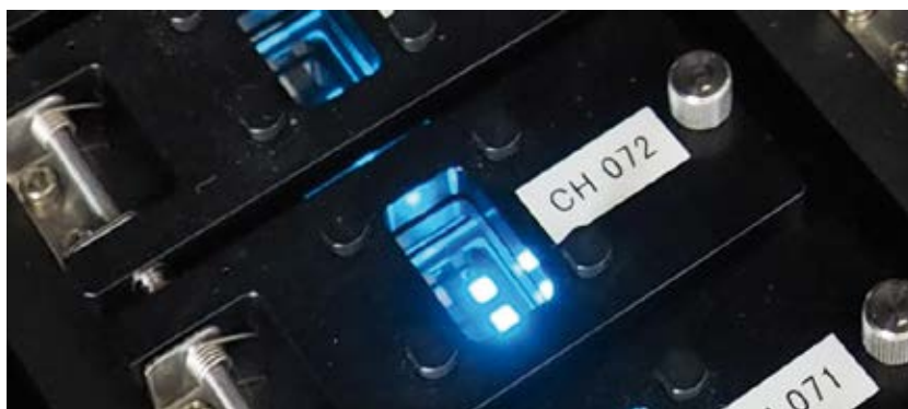
Highly efficient, pure-blue organic light-emitting diodes are tested to measure their lifetime. (Source: Kyushu U.)
