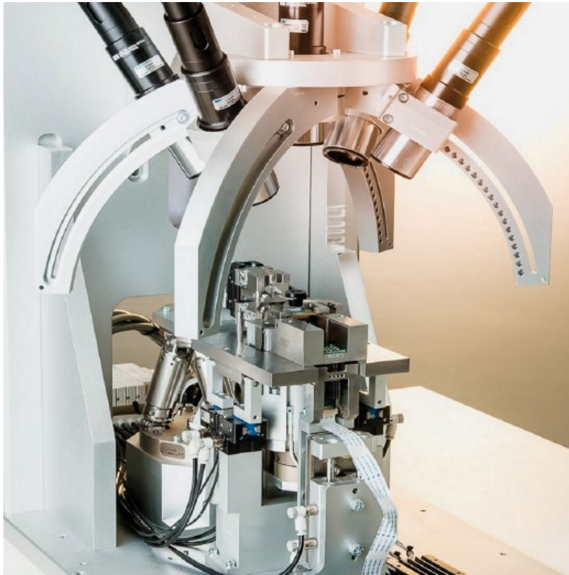
Fig. 2 Active Alignment workstation with flexible collimators setup (top), hexapod and microactuators (bottom rear and center). In this application, an optics group (lens barrel) is actively aligned over a camera chip on a PCB, after which all are held in position by the Position Freezing Carrier (center).
