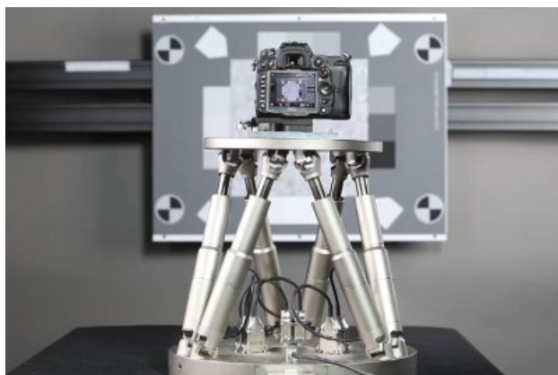
Fig. 2 The H-840 hexapod is designed for the testing of image stabilization systems and certified to CIPA Standard DC-011-2015. (Source: Dxomark)
