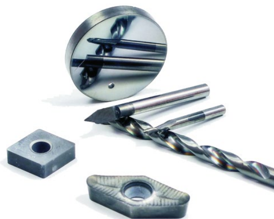
Fig. 4 Hydrogen-free diamond-like coatings reduce tooling wear (Source: S. Weissmantel, Laserinstitut, Hochschule Mittweida)
