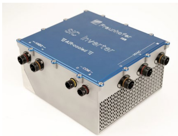
Fig. 2 Innovative heat sink design: the aluminum housing of this new SiC inverter from Fraunhofer-IISB was created in FKM's laser sintering factory. (Source: Fh. IISB)
