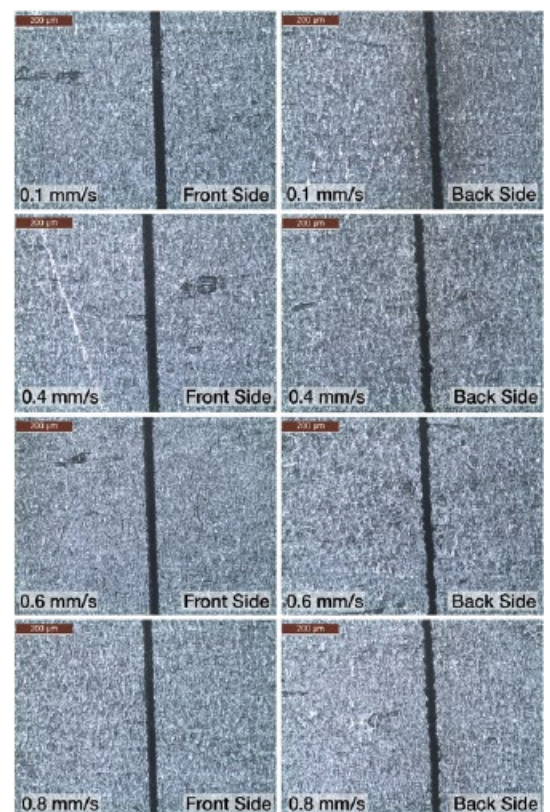
Fig. 3 0.5 mm thick Nitinol cut at different speeds with helium as assist gas and PRF = 100 KHz, pulse energy = 80 \mu J.
