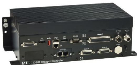
Fig. 4 Digital hexapod controller for easy control: positions are specified in Cartesian coordinates and transformations for the six individual drives take place in the controller. (Source: PI)
