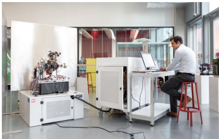
Fig. 3 The UK's first commercially viable quantum accelerometer developed by M Squared and Imperial College London (Source: Thomas Angus, ICL)
