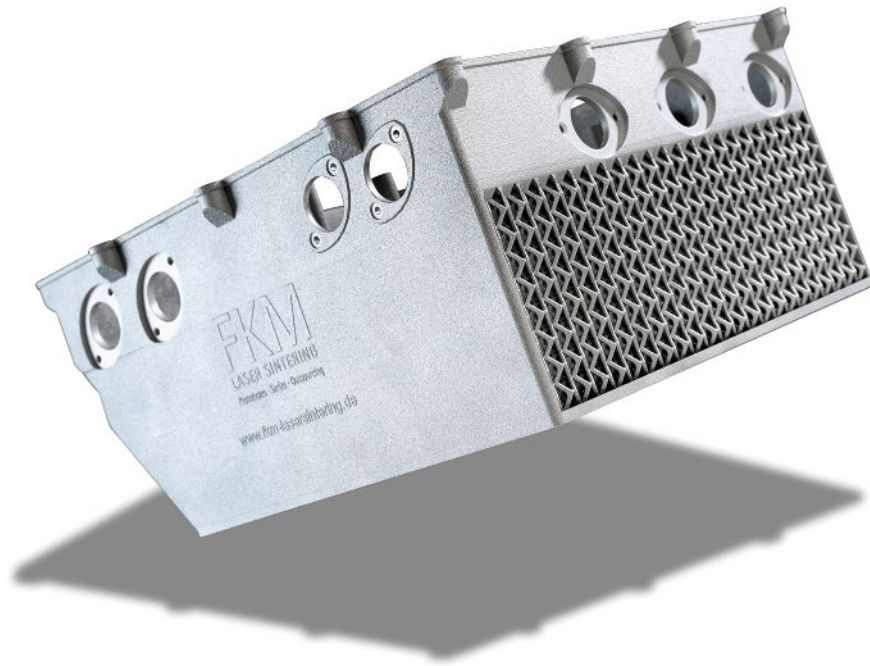
Fig. 1 Laser-sintered Al: housing from FKM for a new, air-cooled SiC inverter developed by Fraunhofer-IISB for use in automotive e-mobility. Complex multi-layer grid structure: metal laser sintering enabled FKM to realize a highly efficient heat sink design for the heat dissipation of the fast-switching SiC inverter. (Source: FKM Sintertechnik)
