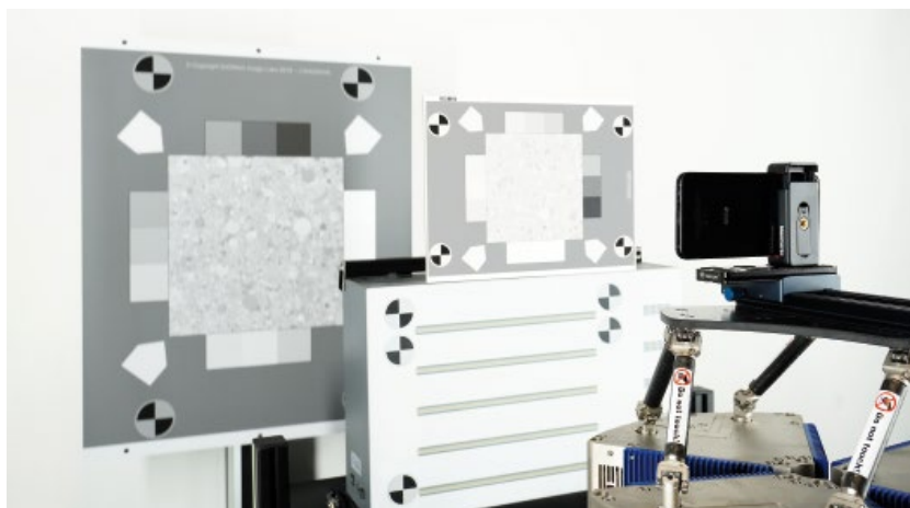
Fig. 1 The new Analyzer is a high-performance and very reliable solution for the measurement of still and video image quality and can be applied in different business sectors. (Source: Dxomark)
