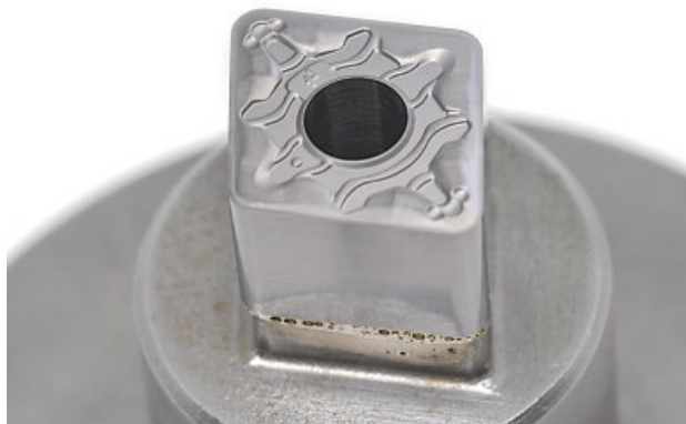
A test customer reduced the production time of sintered inserts (left) from eight hours (with classic EDMing and milling) to two hours (with the KLM E1). Another typical product for the E1: an unpolished stamp (right).
