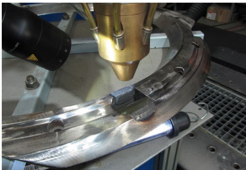
The coating material is applied through concentrically arranged nozzles to the surface area to be treated and melted together with the base material.
