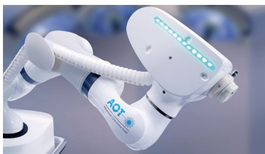
‘Carlo’ can ablate bone layer-by-layer by laser and thus avoids microstructural damage to the bone. (Source: AOT)
