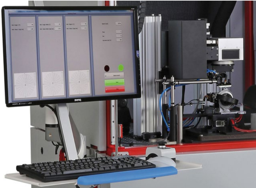
Fig. 1 During the imbalance measurement, the amount of excess mass and the angle are determined in one or two planes. While the impeller stays on the measurement bridge, an x-y scanner directs the radiation of a CO 2 laser to the respective area and the exact amount is ablated. (Source all images: Nanosystec)
