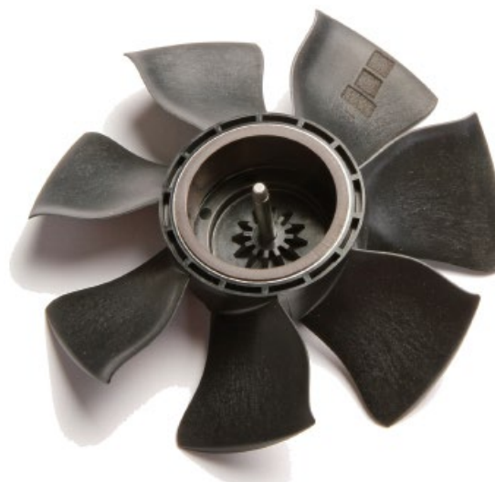
Fig. 3 The ablation areas on this impeller can be seen on one blade. The position and pattern on the fiber-glass enforced plastic are calculated according to the material removal rate of the laser in order to provide a perfectly balanced result.
