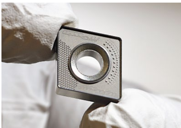
A test customer reduced the production time of sintered inserts (left) from eight hours (with classic EDMing and milling) to two hours (with the KLM E1). Another typical product for the E1: an unpolished stamp (right).
