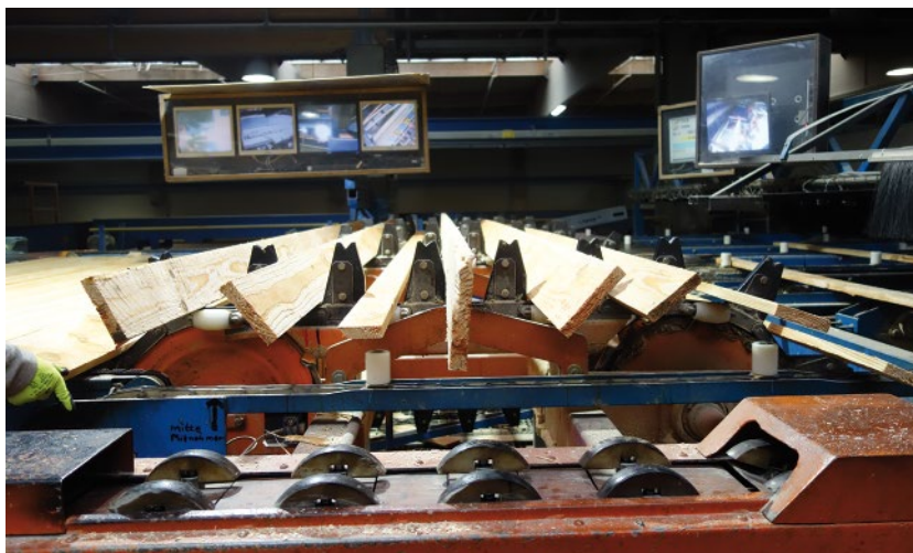
The fine machining is done by a circular saw.
