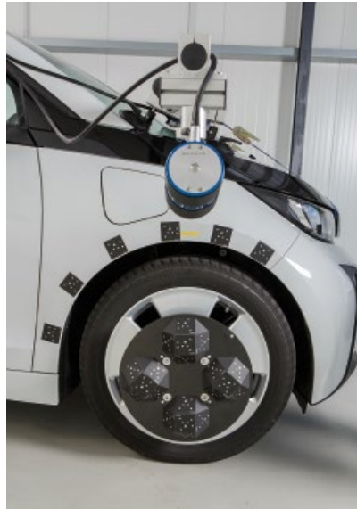
The WheelWatch allows vehicle dynamics testing without mechanical connection between a sensor and the wheel.
