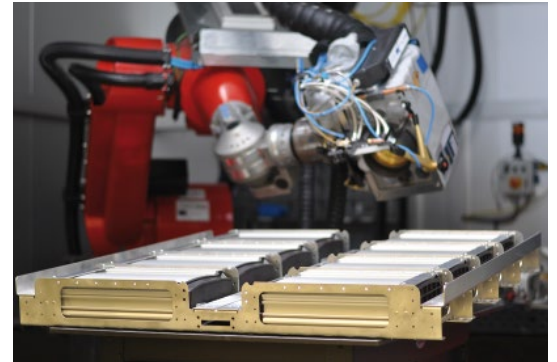
Jigless laser-welded, low-cost battery pack housing made of high-strength aluminum (Source: WZL RWTH)
