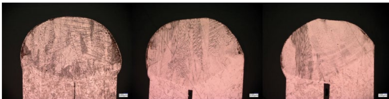
Fig. 3 Bar winding connections are essential for high-fill-factor electric motors, and the blue laser can produce clean hairpin welds such as these 1 mm / 2 mm copper joints.
