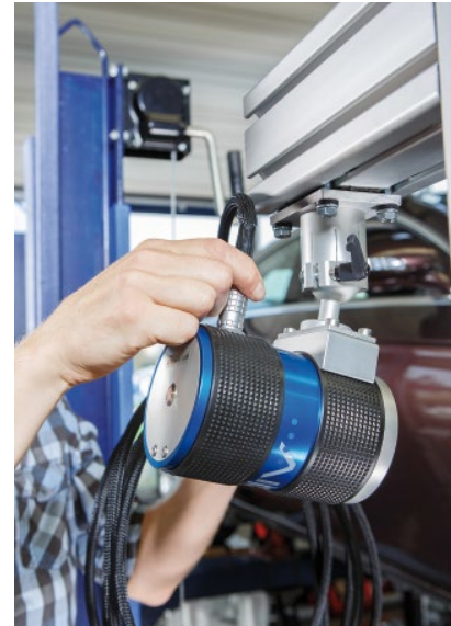
For the measurement of wheel movements, one camera for each wheel is mounted so that the wheel and part of the surrounding fender is visible.
