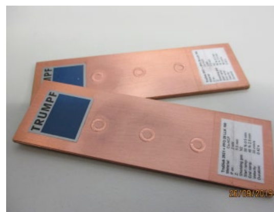
Busbar welding with copper sheets measuring 0.5 by 2 millimeters; an even weld seam surface and consistent penetration depth in a welding time of just 0.42 seconds.
