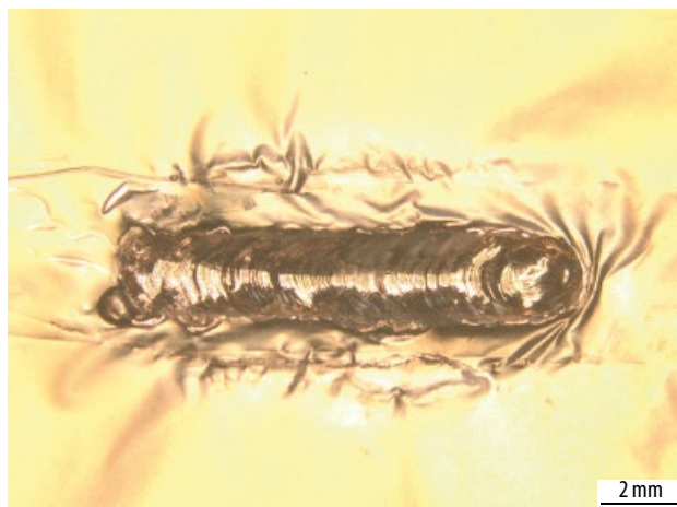
Welding a hundred 6-micrometer battery foils to a 2 \times 0.5 -millimeter copper tab: a large, pore-free bonding surface and a smooth top bead with minimal spatter formation.
