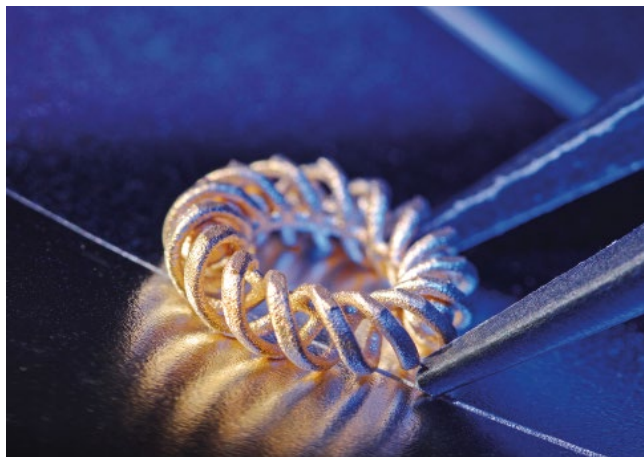
Processing high carbon steels by Laser Powder Bed Fusion (LPBF). (Source: Fh. ILT)
