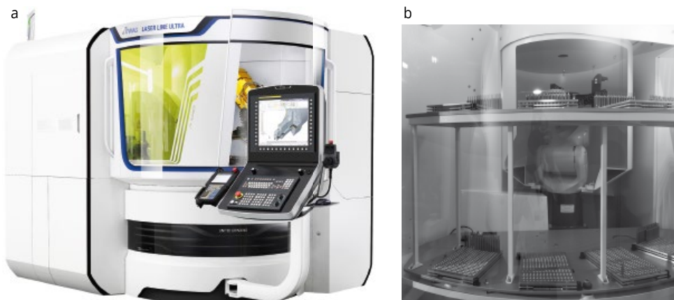
Fig. 4 The EWAG LASER LINE ULTRA machine is an ideal base for highly accurate tool machining, with an integrated automation cell that can be configured as a tool blank storage unit (a). Tool storage within the machine, housing eight pallets: six pallets are used for blank storage of \varnothing = 0.5 - 3 mm blanks and two pallets are used for finished tools (b); sources: Ewag AG)
