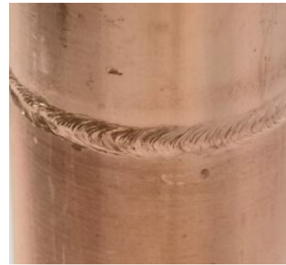
Fig. 3 Deep weld seams achieved by combining green and near-infrared laser radiation. (Source: Siemens)
