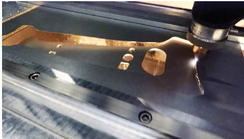
The degree of automation will be a key success factor in the future, especially if several laser cutting heads are involved. Here: high-speed cutting with laser beam. (Source Fh. ILT)
