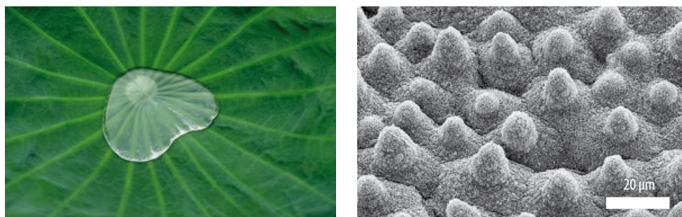
Fig. 2 Image of a lotus leaf, which is naturally superhydrophobic due to the combination of micro- and nano-structures on its surface (left) and SEM picture of the same surface (right, source: W. Barthlott, lotus-salvinia.de)
