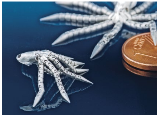
Demonstrator with flexible hinges manufactured using \mu -PBF. (Source: Fh. ILT)
